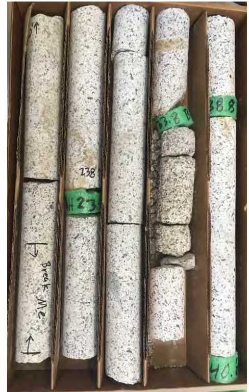
Granitic Bedrock Cores Boring B-09, 20.5 to 40.8 Feet
